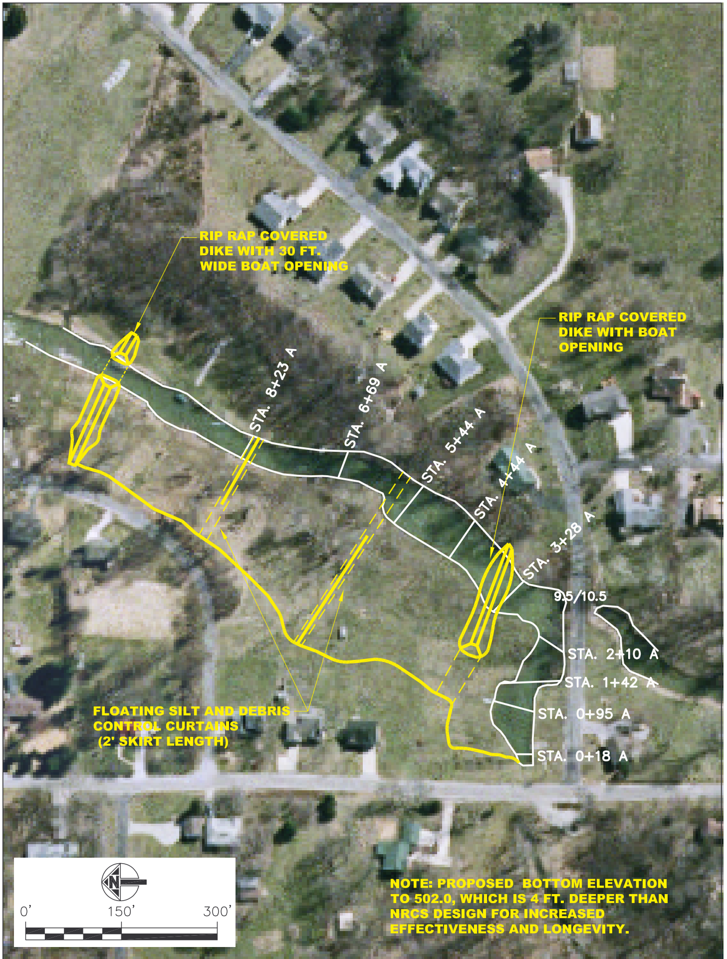
FIGURE 7. NRCS SEDIMENT BASIN WITH ENHANCEMENTS – AREA A
